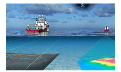
Two Fugro vessels supported the project, completing approximately 200 days of surveys and more than 10,000km of survey lines within the 684km<sup>2</sup> project area. The geo-data collected provides crucial insights into the seabed and sub-surface conditions, enabling installers to make informed decisions on turbine and export cable placement.
